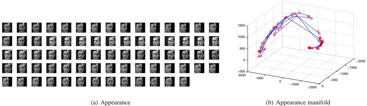
Figure 4. A typical face track obtained using our algorithm. Shown are (a) the original images are detected by the face detector (rescaled to the uniform scale of  $50 \times 50$  pixels) and (b) as points in the 3D principal component space with temporal connections.
