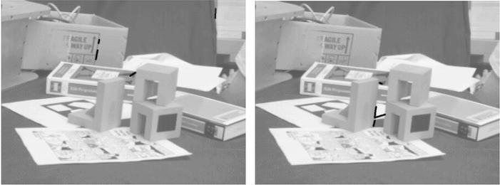
Figure 8: This figure shows two groups of black lines which were found by the algorithm to be coplanar, but do not represent real planes in the scene.
