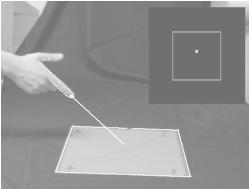
Figure 5: Stereo views of a pointing hand. The two views are shown side by side. In each view an active contour is tracking the hand. The inlaid square is a representation of the indicated point in working plane coordinates.
