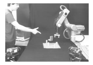
Figure 4: **Arrangement of the stereo cameras, table and robot.** The cameras view the robot, workspace and operator's hand from a distance of about 1.6m.
