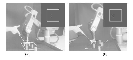
Figure 8: Gestural control of robot position for grasping, seen in stereo. The robot gripper servos to the position indicated by the pointing hand; here it is being instructed to align itself with the small wooded block to be grasped. The four reference points (white rectangle) were defined by the robot's gripper in a plane 50mm above the table.
