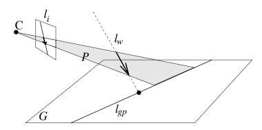
Figure 1: Relation between lines in the world, image and ground planes. Projection of the finger's image line  $l_i$  onto the ground plane yields a constraint line  $l_{gp}$  on which the indicated point must lie.
