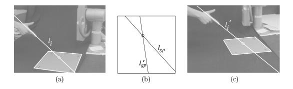
Figure 2: **Pointing at the plane.** By taking the lines of pointing in left and right views (a, c), transforming them into the canonical frame defined by the four corners of the grey rectangle (b), and finding the intersection of the lines, the indicated point can be determined; this is then projected back into the images.
