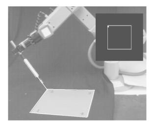
Figure 7: Mechanical pointing device used to test the accuracy of our system. We aligned the rod with known points on the workspace, and recorded its coordinates as recovered by the vision system.
