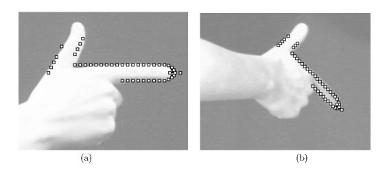
Figure 3: The finger-tracking active contour, (a) in its canonical frame (b) after an affine transformation in the image plane (to track a rigid motion of the hand in 3D). It is the index finger which defines the direction of pointing; the thumb is observed to facilitate the tracking of longitudinal translations which would otherwise be difficult to detect.
