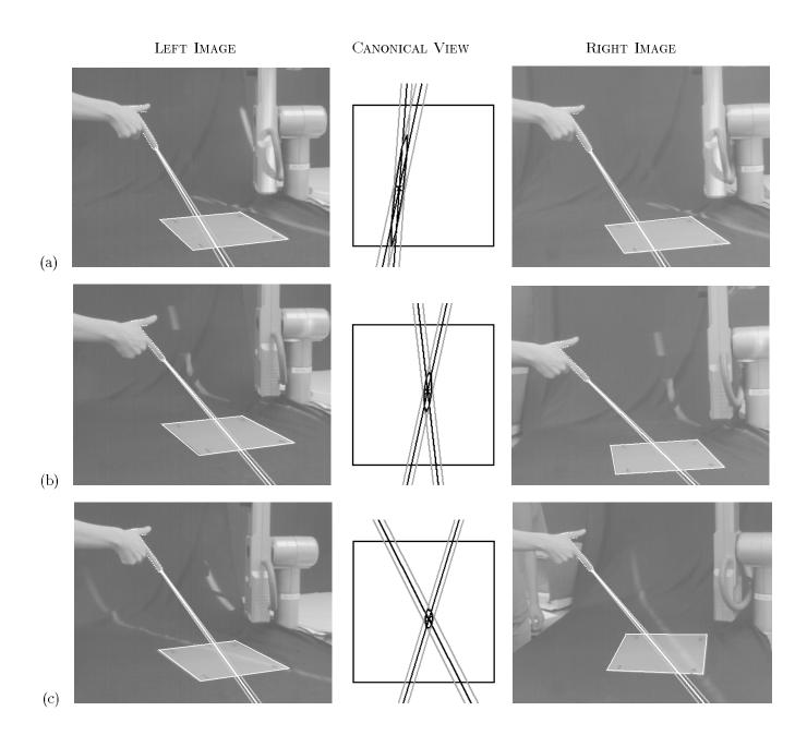
Figure 6: Indicated point uncertainty for 3 different camera configurations.  $2\sigma$  bounds for the pointing lines, their projections into working plane coordinates, and error ellipses for the indicated point, when the angle between stereo views is (a)  $7^{\circ}$  (b)  $16^{\circ}$  (c)  $34^{\circ}$ . The uncertainty is greatest when the camera angle is small and the constraint lines nearly parallel.
