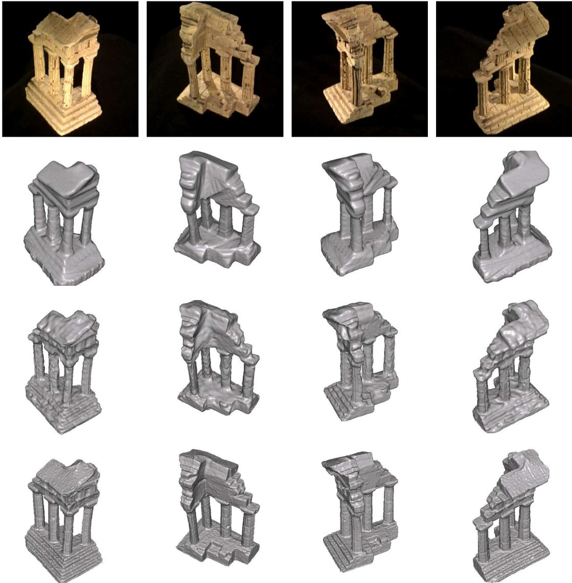
Fig. 5. **Castor and Pollux (Dioscuri) temple sequence.** First row: Four of the input images. Second row: Visual hull obtained from silhouettes. Third row: Results obtained with the original Volumetric Graph-cuts formulation of [29]. Fourth row: Results obtained with the method presented here. The occlusion robust photo-consistency metric greatly enhances the detail of the reconstruction.
