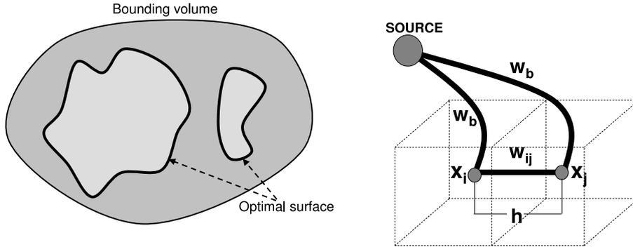
Fig. 3. **Surface geometry and flow graph construction.** On the left: a 2D slice of space showing the bounding volume and the optimal surface inside it that is obtained by computing the minimum cut of a weighted graph. Note that complicated topologies such as holes or disjoint volumes can be represented by our model and recovered after optimisation. On the right: the correspondence of voxels with nodes in the graph. Each voxel is connected to its neighbours as well as to the source.
