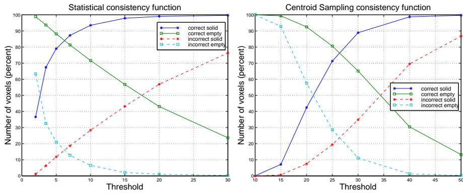
(b) These two graphs show the effect of corrupting the synthetic images with Gaussian noise ( $\sigma=10\%$ ). The centroid sampling method performs considerably worse than the statistical method in this case. Notice how the two *correct* curves cross at 85% and 75%. (not 85% and 80% as they did in figure 9(a)).
