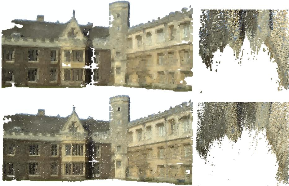
Figure 6: Space carving using the statistical consistency function. The top two images show a reconstruction of the Great Court image sequence with  $128^3$  voxels. The important thing to notice is that the windows have been correctly reconstructed, in contrast to figure 4. The lower two images use  $256^3$  voxels.
