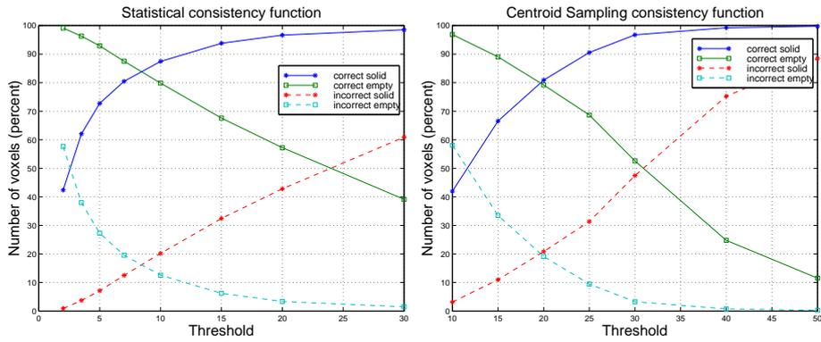
(a) These graphs were generated from synthetic data, with no added noise. Compare the intersection of the two *correct* curves which occur at 85% and 80%. Notice how the statistical method performs slightly better due to better handling of voxel aliasing.
