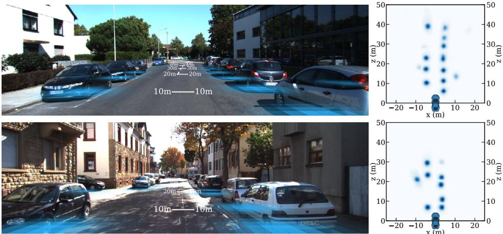
Figure 4: Examples of confidence maps generated by our approach, which we visualize both in birds-eye-view (right) and projected onto the ground plane in the image view (left).
