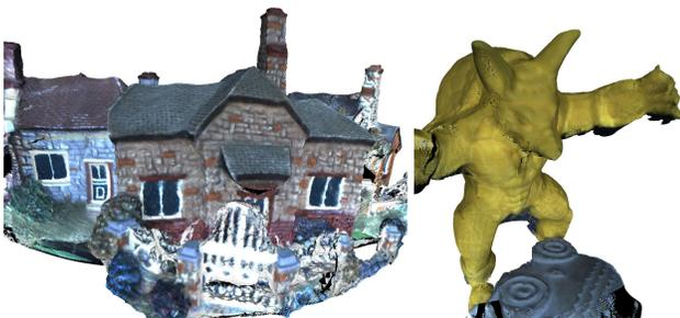
Figure 13. Albedo-mapped reconstruction of the 2 multi-object datasets. The albedo is calculated using simple least squares on Equation (2) using the final geometry estimate (along with occlusion/shadow maps). Black albedo regions signify that this particular part of the surface is not visible in any image.
