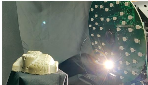
Figure 1. Our Photometric Stereo setup consists of 52 LEDs placed within the same plane of the camera image. 14 objects have been acquired at a distances 10-30cm in order to capture full near-field effects. The materials of the objects provide a variety of diffuse and specular reflections, including wood, aluminium, plastic, etc.
